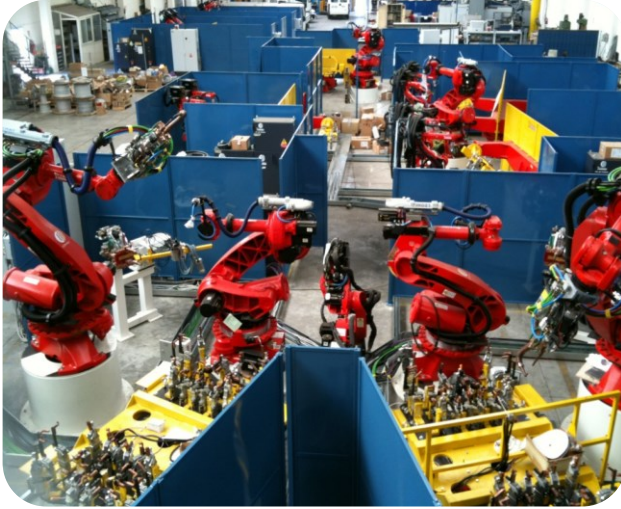
Fiat 846 Front suspension cross member welding system
