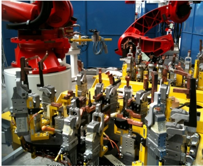
Tool for welding CO2 seat elements
