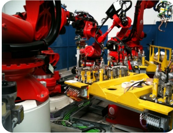
Fiat 846 Front suspension cross member welding line
