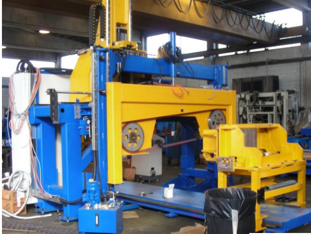
Beam cutting, drilling, butting and marking system
